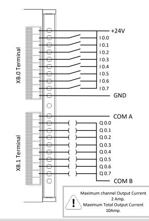
**Digital Input and Relay Output Connections**
